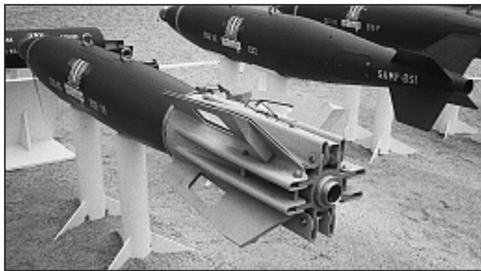
BL EU2FR fragmentation bomb with a US BSU-86B retarding tail unit on the left, and on the right a BL EU2P with a standard BS1 low-drag tail unit (Peter Humphris) 0504927
