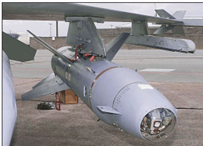
A Have Lite (Popeye 2) missile during US testing, carried by an F-16 (Rafael) 1120836
