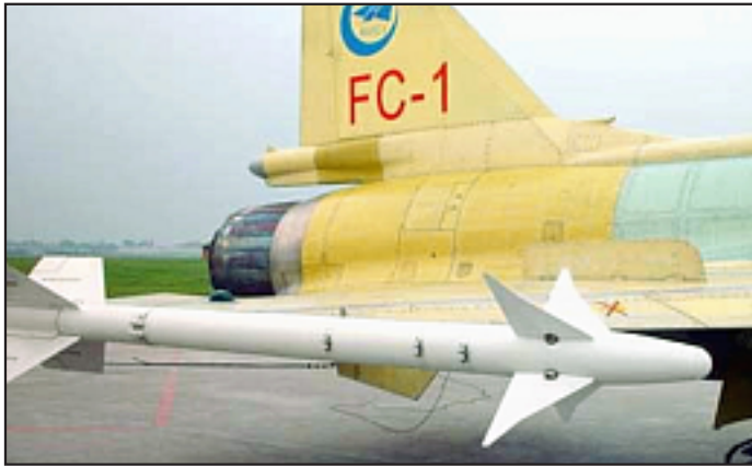
A PL-5E missile carried by one of the prototype CATIC FC-1 (JF-17) light fighter aircraft (via Robert Hewson) 0558914
