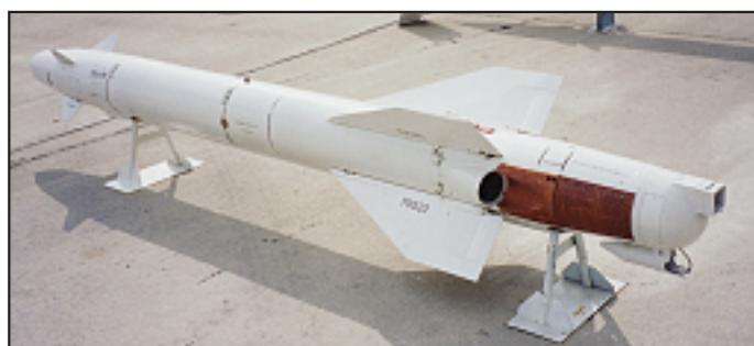
The command guidance radio antenna for the Kh-25MR is fitted to the missile's tailcone (Christopher F Foss)
