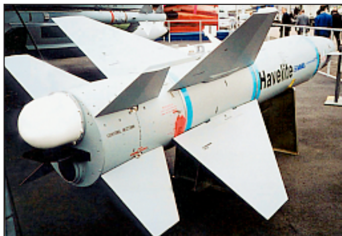
A view of the Have Lite (Popeye 2), showing the datalink antenna repositioned above the motor nozzle (Peter Humphris) 0092777
