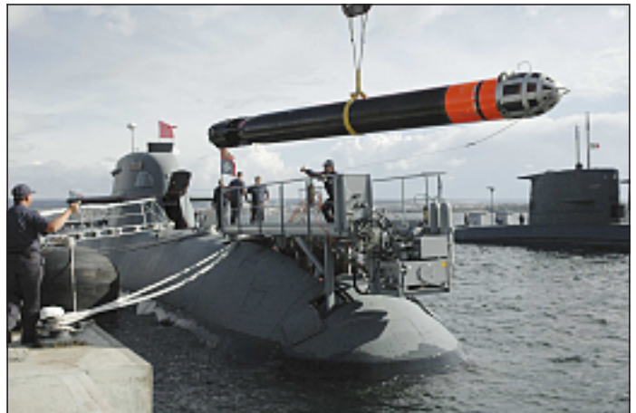
A DM2 A4 torpedo being loaded in to an Italian Todaro-class (Type 212A) submarine prior to a trial (ATLAS Elektronik)
