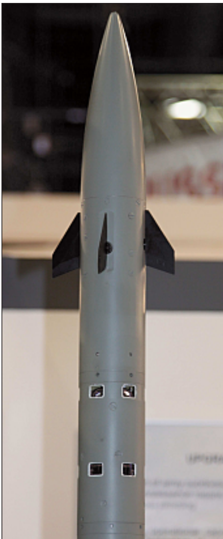
The Sosna-R missile showing the optical ports for the laser proximity fuze (Miroslav Gyürösi)
