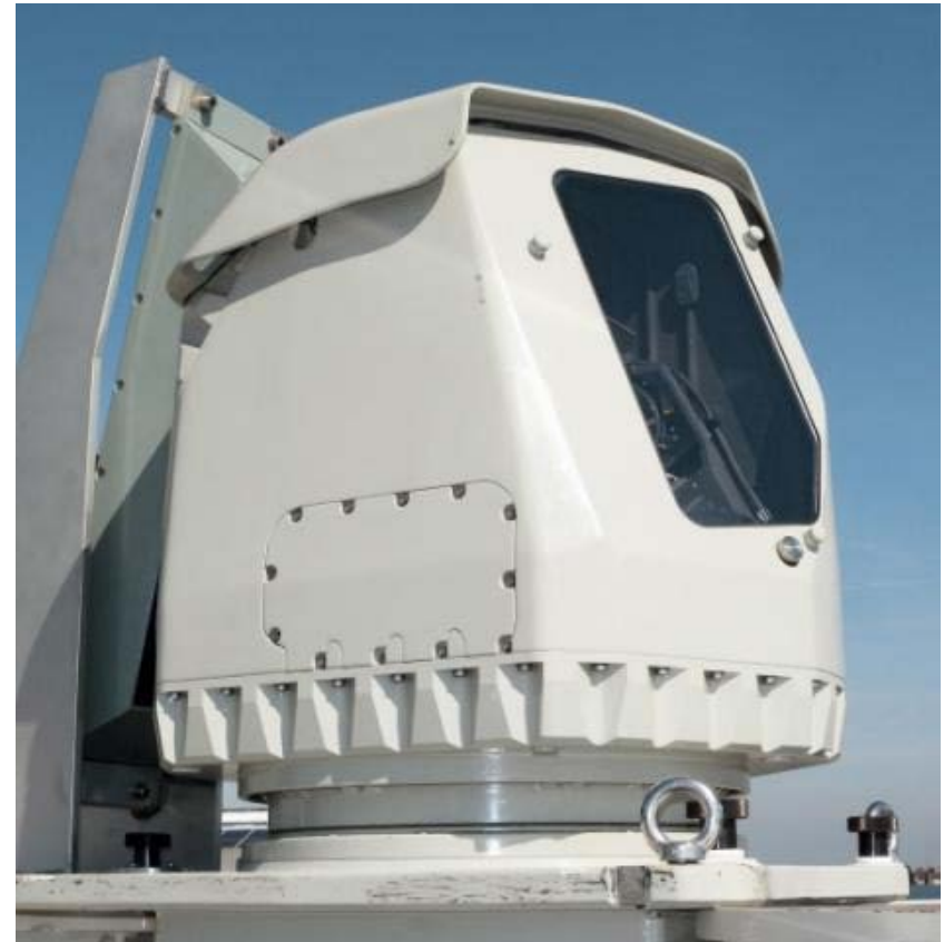
The sensor head of VAMPIR-NG, in production for the Russian Mistral-class BPC and the Royal Australian Navy (image © Sagem)
