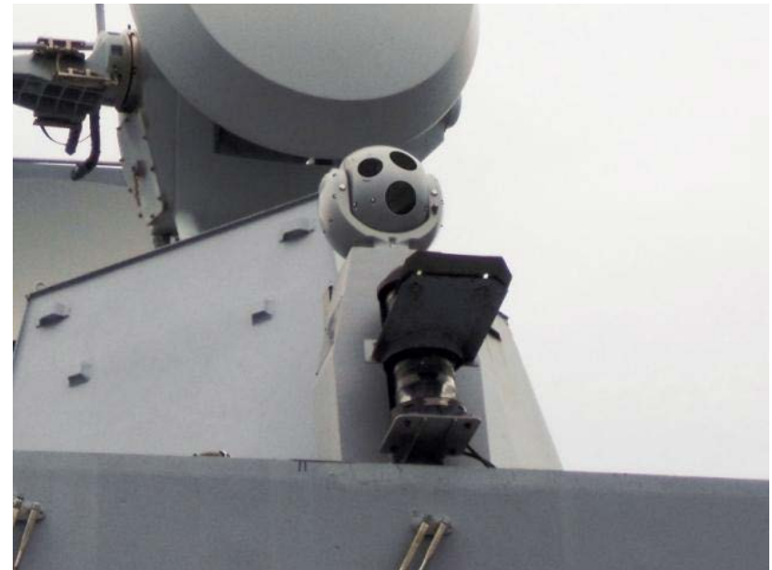
The Janus-N EO/IR system – shown here on an Italian Comandante-class patrol vessel – has now been ordered by Malta (image © Selex Galileo)
