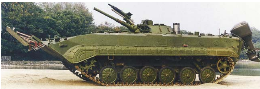
Chinese WZ501 IFV modified for amphibious operations with new, larger trim vane on front of hull and large outboard motor at rear (image © NORINCO)
