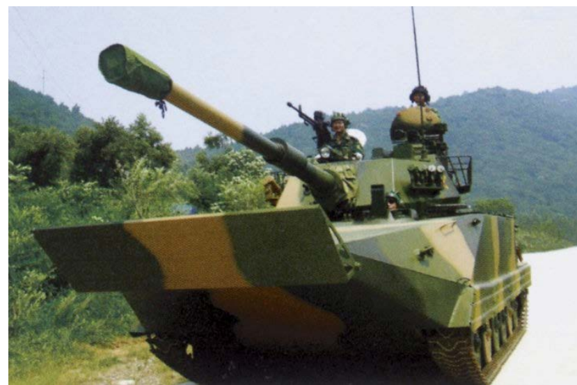
The upgraded Type 63A light amphibious tank features a new turret and greater buoyancy, shown here with trim vane extended at the front of the hull for amphibious operations (image © China Xinshidia Company)
