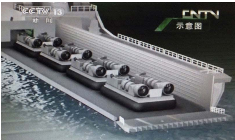
This cutaway shows the internal well dock arrangement of the Type 071 LPDs, with the dock running roughly two-thirds of the ship's length (image © CCTV, via R Foster)
