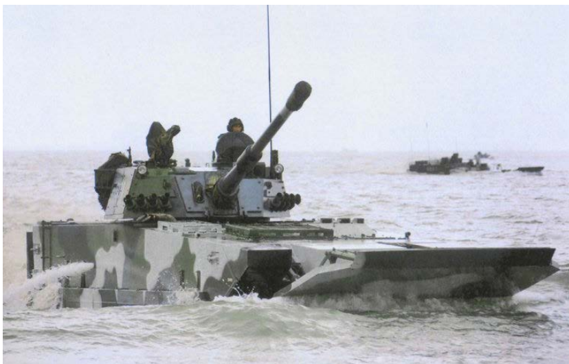
The ZTD-05 amphibious direct-fire vehicle armed with a 105 mm gun coming ashore during amphibious operations. (image © INA)
