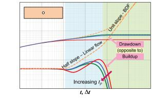
Infinite-Acting Homogeneous Reservoir:
