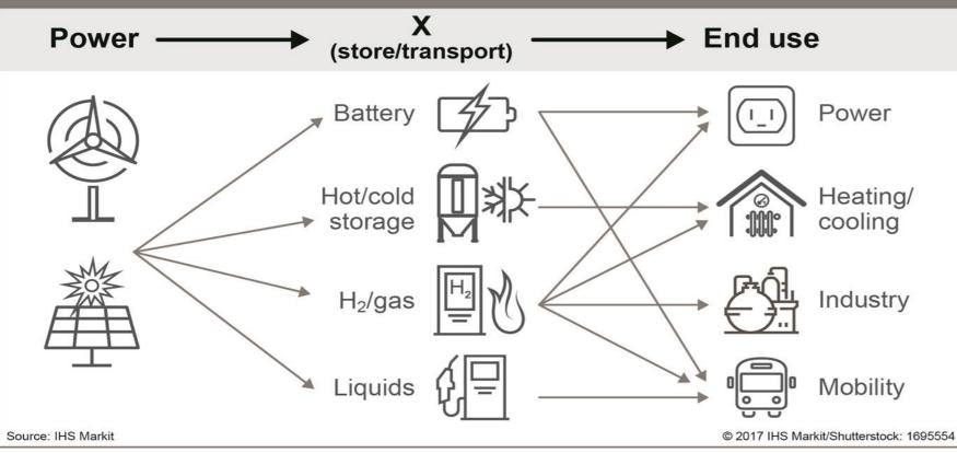
Power to hydrogen to power is in direct competition with batteries for intra-day balancing
