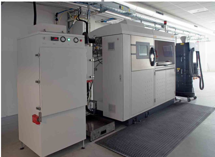
This direct metal laser sintering (DMLS) 3D printer employs an additive manufacturing technique that uses a Ytterbium fiber laser fired into a bed of powdered metal.
